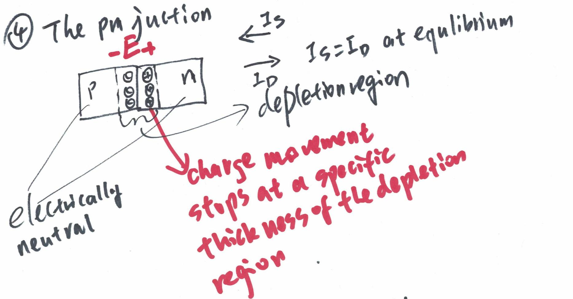
⑤ current driven by the Electric field :  $I_S$  (drifting current)
