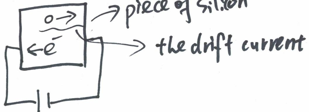
$V_{p\text{-drift}} = \mu_p \cdot E$  → intensity of the electric field
