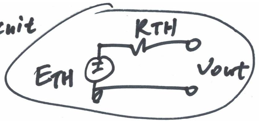
$$R_{TH} = R_3 \parallel (R_1 \parallel R_2)$$
