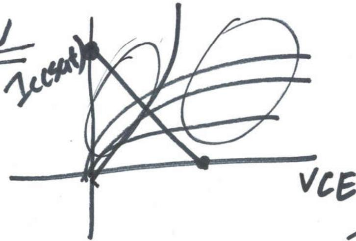
$$I_{C(sat)} = \frac{V_{CC} - 0}{R_C}$$
