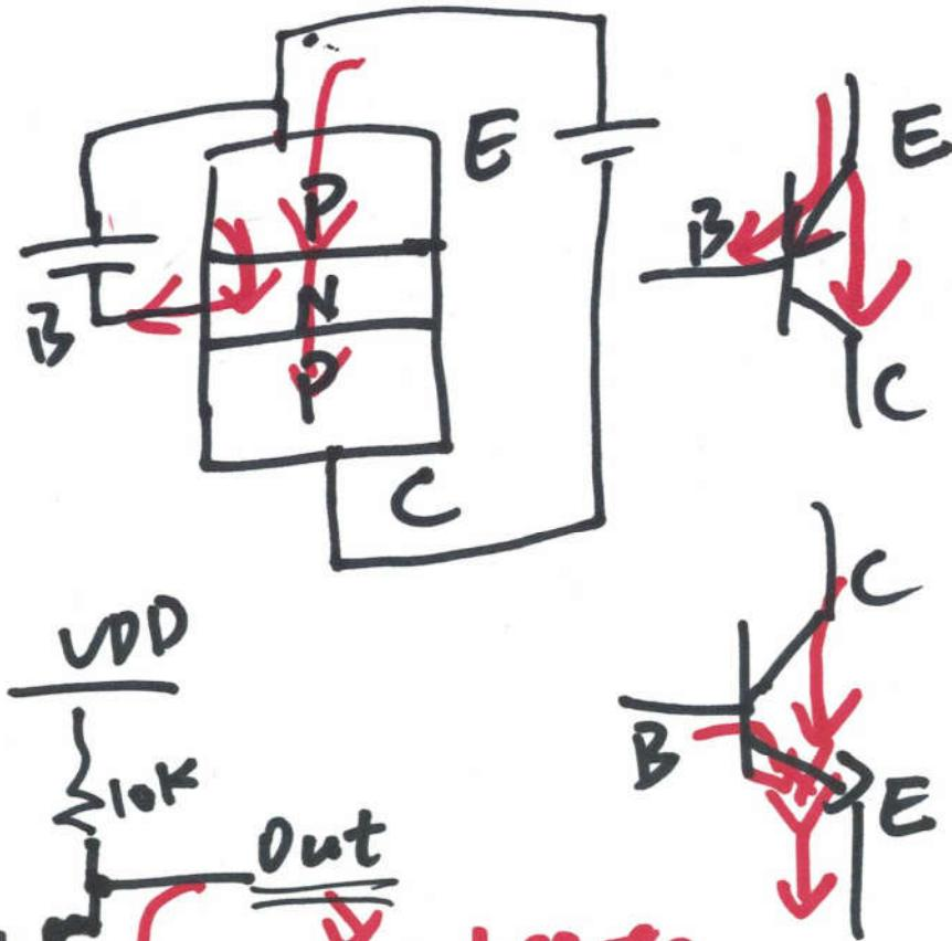
$I_{in}$  High  $V_{DS}$  very close to GND
